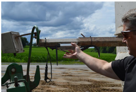
A precision feeding system transponder mounted on a feeding wagon. It relays the weight of each ingredient as it is loaded into the wagon to enable a highly accurate recipe.
