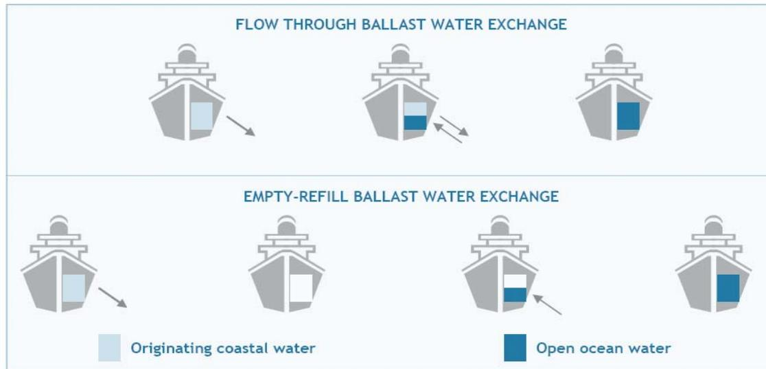
**Fig. 21. The two forms of ballast water exchange: flow through and empty-refill. A flow-through exchange continuously pumps ocean water into ballast tanks, forcing coastal water out. In an empty-refill exchange, a ballast tank filled with coastal water is completely flushed and refilled with ocean water.**
