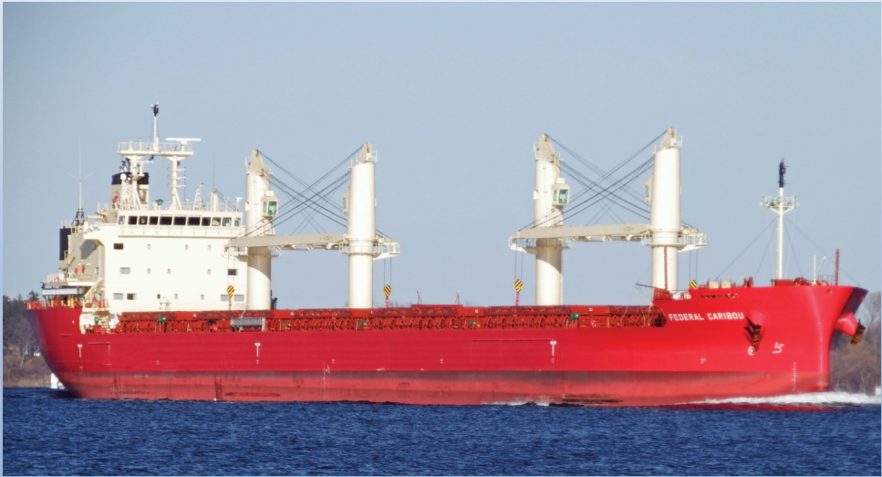
Federal Caribou , built by Fednav Limited, represents a new class of Great Lakes “salties” designed to include a ballast treatment system. The BallastAce treatment system by JFE Engineering is based on chlorine and filtration.
